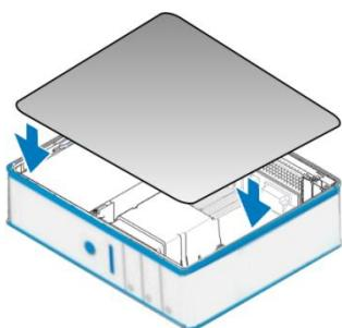
Re-attach cover for the computer and reconnect the power supply.
