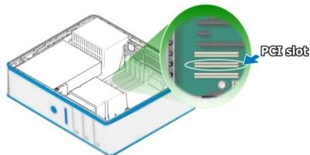
Select an empty PCI or PCIe slot.
