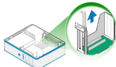
Remove the screw holding the cover for the PCI slot in place and then remove the slot cover from the PC. Ensure that you do not misplace the screw.
