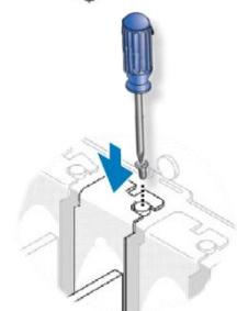
Screw the mounting bracket screw into the new PCI or PCIe card bracket to secure the card in place.
