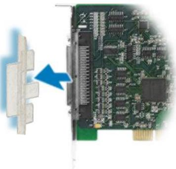
Remove the connector cover form the card.
