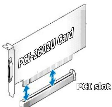
Align the contacts of the card with the open slot on your motherboard and carefully insert your card into the PCI or PCIe slot.
