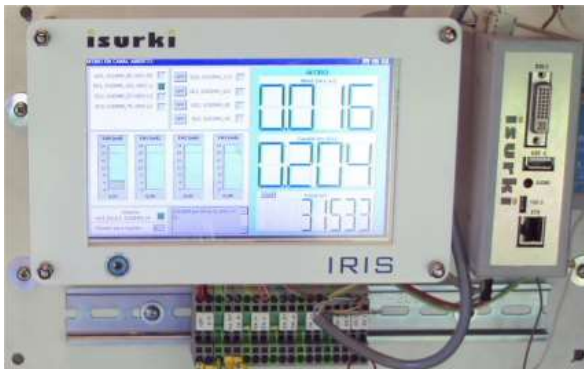
IRIS BOX PC unit with a 7" IKUS touch screen in an open channel flow rate calculation and telemetering real application
