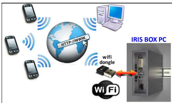
WIFI connectivity through the USB dongle.
