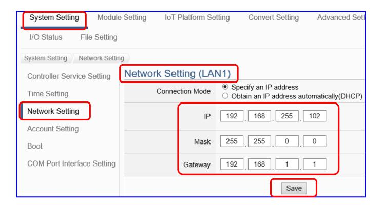
**5.** Save the IP setting, restore the PC original IP settings, and type the **new IP** in the browser as step-3 to login the Web UI of UA-5200. And then configure user's UA project.
