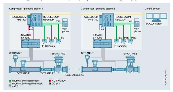
The RUGGEDCOM RSG920P is ideal for the field level where growing demands for Ethernet connectivty exists.
