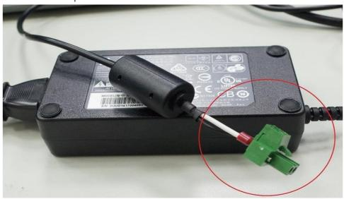
2. Connect the 3-pin male plug of the power cord to an electrical outlet.
