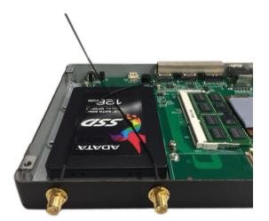
6. Insert the ring onto the antenna jack end of the cable.
