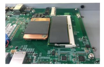
3. Open the bottom cover for installing the 2nd SO-DIMM memory module.
