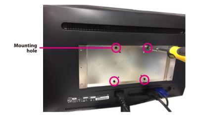
2. Secure the system to the VESA mount bracket with screws.
