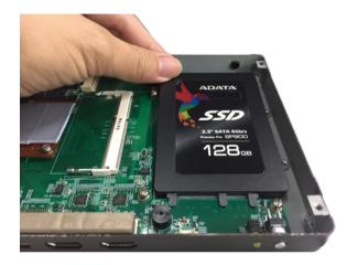
3. Then use screws to secure the drive from the bottom of the chassis.
