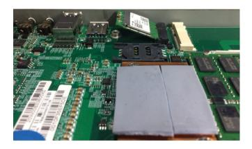
4. Secure the module with mounting screws and attach one end of the RF cables onto the module.
