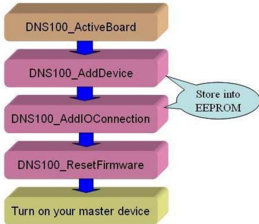
Figure 4.2.1 Slave Configuration Diagram
