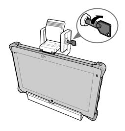
While supporting the R11 tablet PC with one hand, push the latch backward until it fully disengages.
