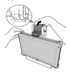
3. Remove the R11 tablet PC from the docking cradle.
