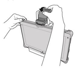
3. Fully push the latch bar into position to ensure the latch is tightly secured.
