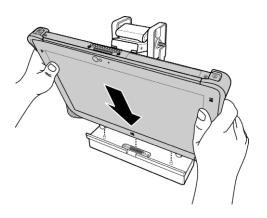
Secure the R11 tablet PC by pulling the latch forward until a "click" is heard and the latch is fully engaged.
