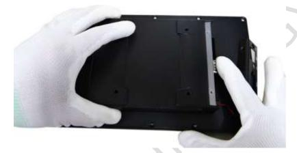
5. Remove the screw of Mini-PCIe Slot.
