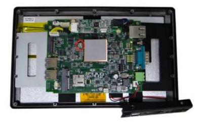
Plug M.2 2242 Storage on M.2 Slot and lock the screw back. 6.
