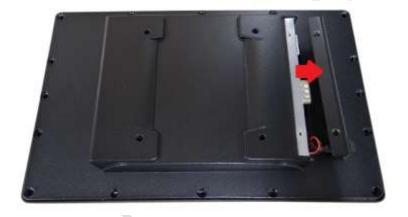
Pull up and remove the rear cover.
