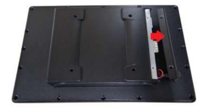
Pull up and remove the rear cover.
