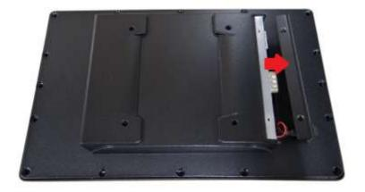
4. Pull up and remove the rear cover.
