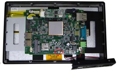
6. Plug Mini-PCIe Module in the slot and lock the screws.
