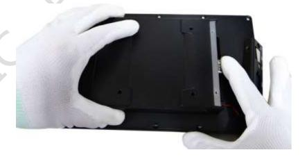
5. Remove the screw of M.2 Slot.
