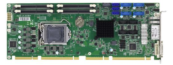
ROBO-8114VG2AR is based on Intel® C246 chipset with workstation processor or Intel® Q370 chipset with desktop level processor. Built with flexible PCI express expansions, ROBO-8114VG2AR is suitable for Medical, Industrial Automation, and Digital Signage applications.
