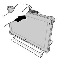
3. Ensure the R11 tablet PC is tightly secured to the docking cradle.
