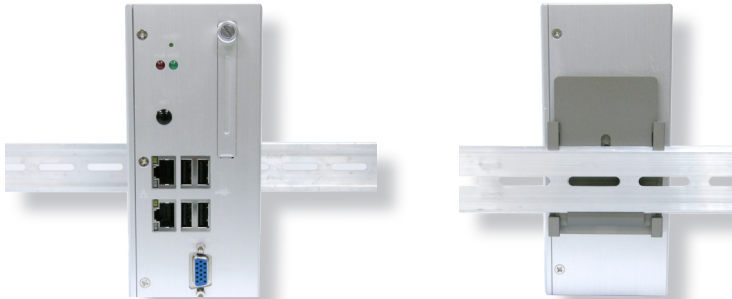
Computer mounted on DIN-rail
