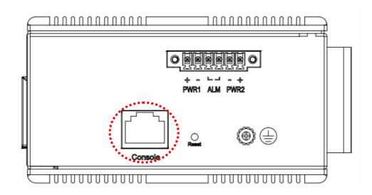
To connect the host PC to the console port, a RJ45 (male) connector-to-RS232 DB9 (female) connector cable is required. The RJ45 connector of the cable is connected to the CID port of IVS-500; the DB9 connector of the cable is connected to the PC COM port. The pin assignment of the console cable is shown below:
