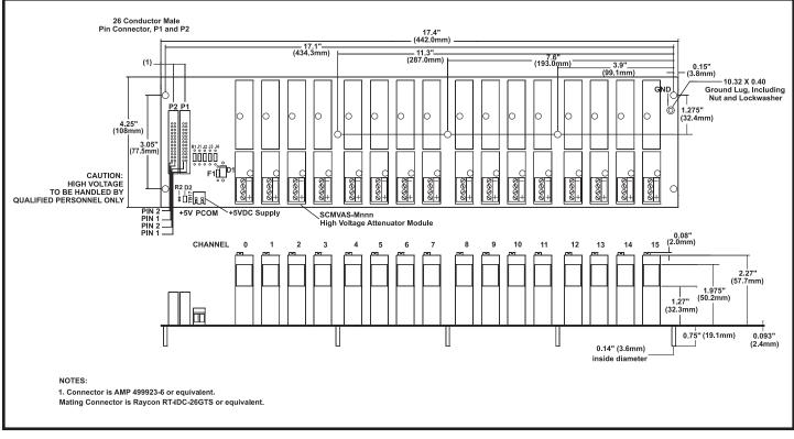
Figure 4: SCMVAS-PB16 Analog I/O Backpanel
