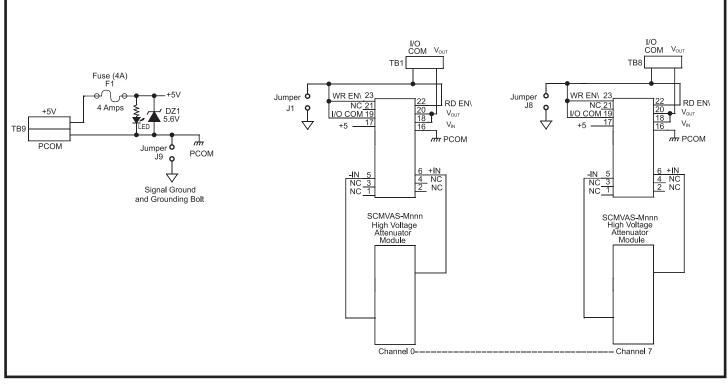
Figure 3: SCMVAS-PB8 Schematic
