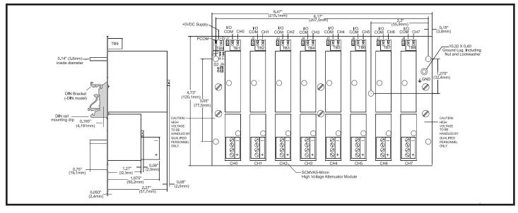
Figure 2: SCMVAS-PB8 Analog I/O Backpanel
