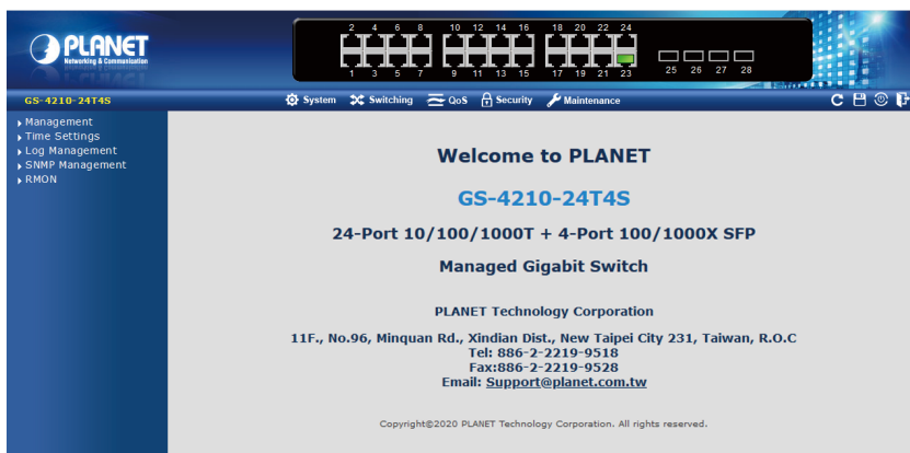
Figure 4-3: Web Main Screen of Managed Switch
